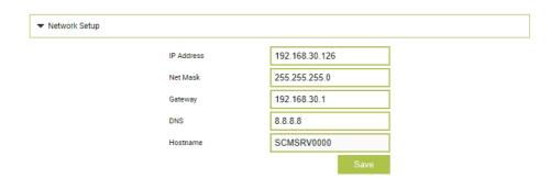
The parameters of the SBC's network configuration can be specified in this section by setting which IP address the control system's web page will be listening to.
